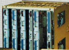
34 Mbit/s Office Repeater
