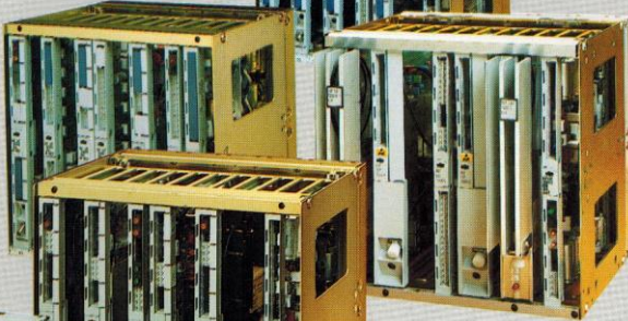
140 Mbit/s Office Repeater 850 nm multi-mode version.
