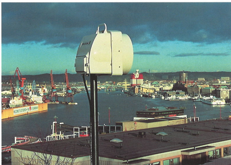
Mini-Link microwave transmission systems can be installed quickly and easily, as an alternative to running cable or fibre.
