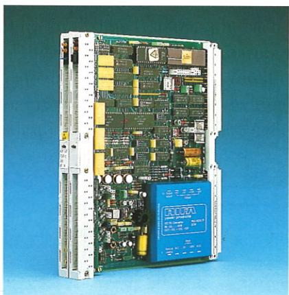
The ZAN 011 protection switching system can switch a 2 or 8 Mbit/s signal to an alternative path within 10ms of detecting an alarm.
