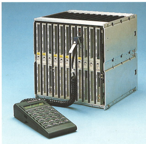
The ZAE 103 01 subscriber multiplexer, complete with programming unit. It can be used as a remote or central subscriber multiplexer.
